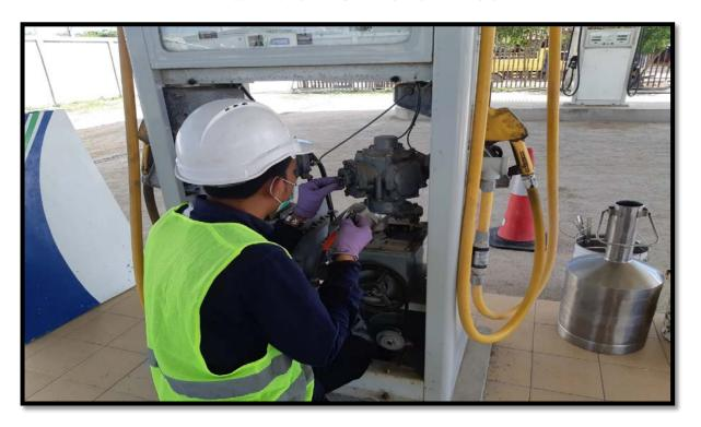
FIGURE 28: VERIFICATION AND CALIBRATION ACTIVITY AT ALBATROS FFS IN BAUCAU
