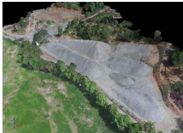
FIGURE 50: DRONE MAPPING AND STOCKPILE VOLUMETRIC SURVEY
