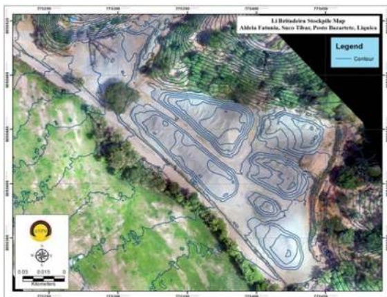
FIGURE 50: DRONE MAPPING AND STOCKPILE VOLUMETRIC SURVEY
