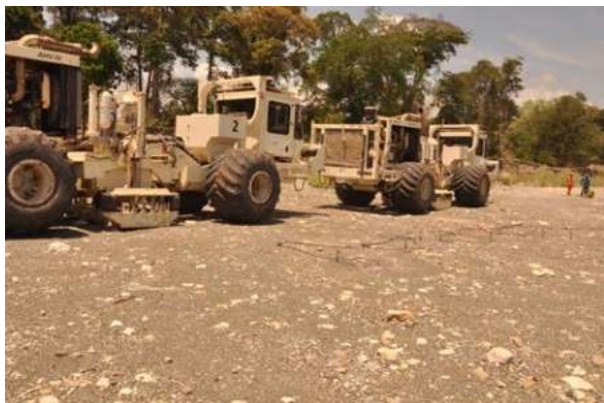
FIGURE 9: VIBROSEIS SEISMIC SURVEY ACTIVITIES
