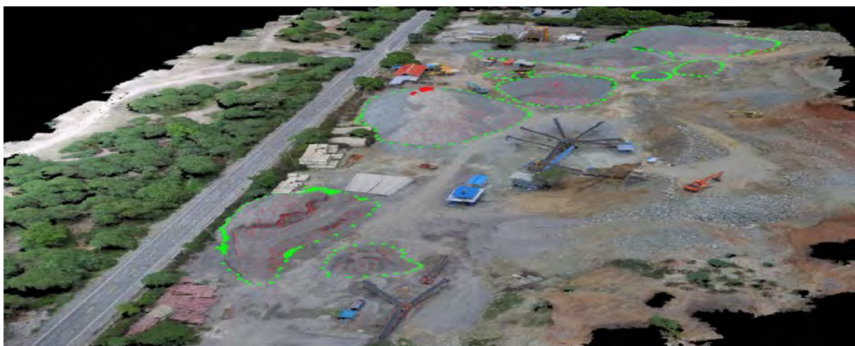
FIGURE 33: PROCESSED DRONE IMAGE FOR STOCKPILE VOLUMETRIC CALCULATION
